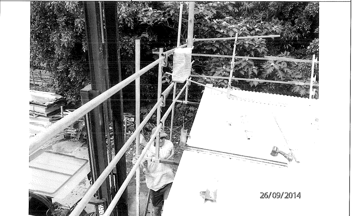
Figure 4 Fascia Bracket System with Pendulum in position Pendulum in position before impact testing.
