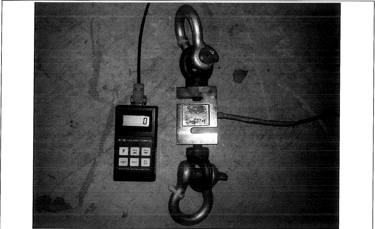
Figure 5 Load Cell and display Load cell used to apply and measure static forces.
