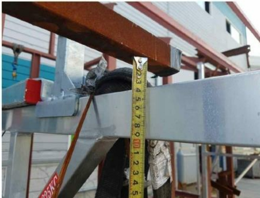
Figure 7- Deflection 40mm measured at 339 KGF
