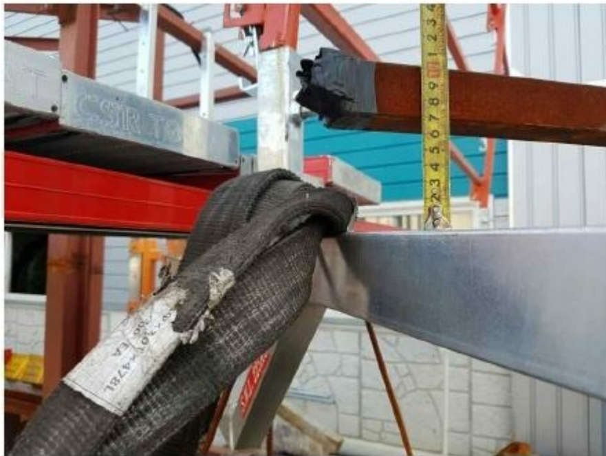
Figure 9- 70mm deflection measured at 2.2meter Corner Arm
