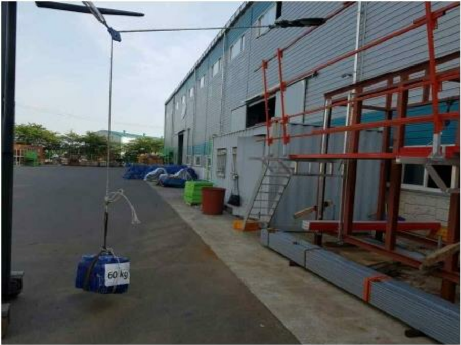
Figure 10- Static Load 60kgf applied at center of Top Rail Span,
