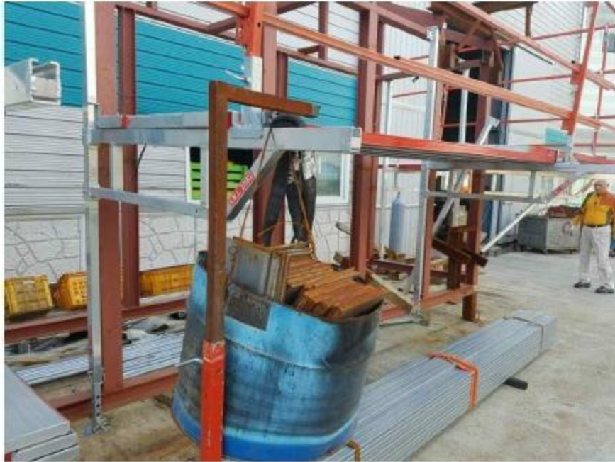
Figure 6- 1.5 meter Platform Arm Static Loading 339 KGF
